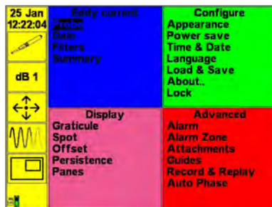
Simple single screen menu showing four user assignable soft keys and one "last item used" soft key
